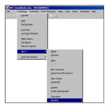
On the **HEC-1 ROUTING DATA** form, check the custom check boxes to the right of the **'Steps'** field for all the return periods. This allows you to enter an initial step value into the current routing card. Enter initial step values into the **'Steps'** field. Now, uncheck the custom check boxes and press **'Save'**. Repeat for every routing card or record. When finished, press **'OK'** to close the **HEC-1 ROUTING DATA** form.
