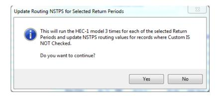
After the last HEC-1 run is completed, the NSTPS values for the routing cards will be updated. Press 'OK' to close the HEC-1 ROUTING DATA form.
