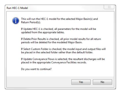
Afterwards, you can view the model results by clicking the 'Results' button on the Run HEC-1 Model form. Alternatively, you can also view the results from 'Hydrology > HEC-1 > Flow Summary'.
