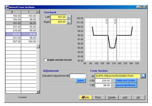
Compare the geometric data on the **NATURAL CROSS SECTIONS** form against the tabulated data listed below. Make necessary data edits or adjustments on the form, if necessary. Click **OK** to close the form.
